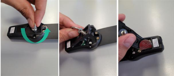
2. Insert the new battery and put the cover back on, turning the ring 90° clockwise.
